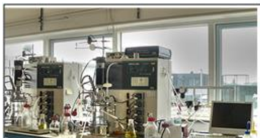
Fig. 23.14 Production of Recombinant Buffalo Chymosin in 10L fermenter
