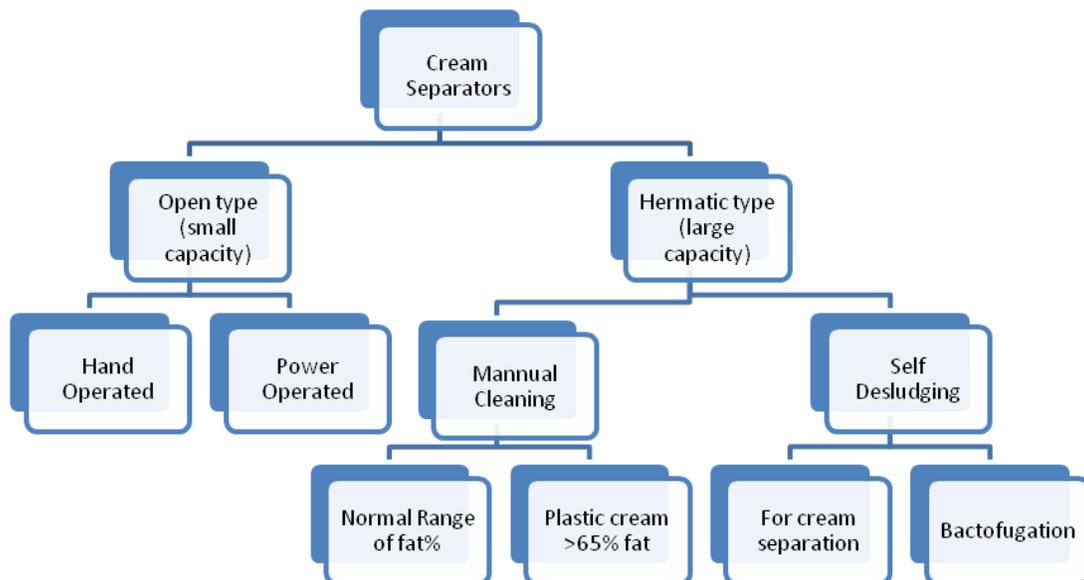
Fig.11.1 Types of centrifuges
