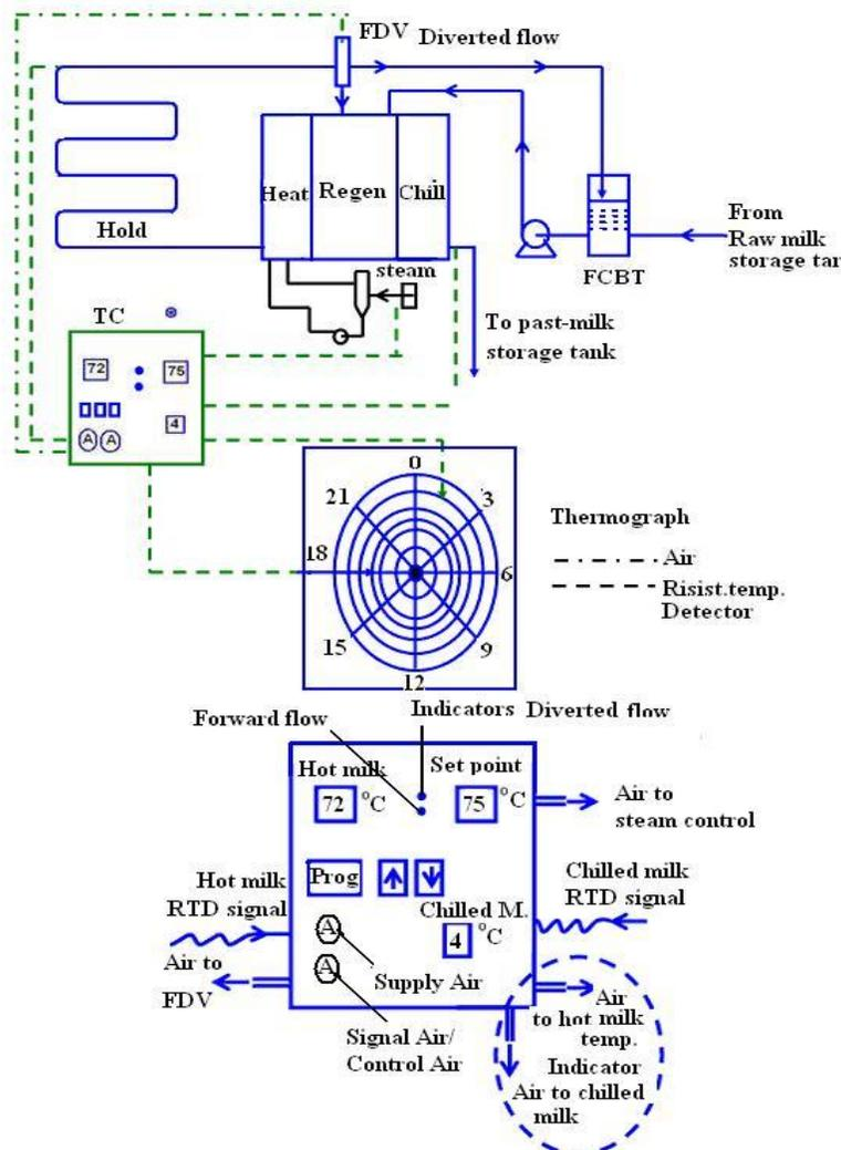
Fig.18.1 Pasteurizer controls
