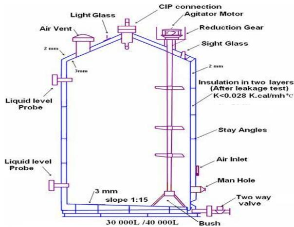
**Fig.4.2 Vertical storage tank**
