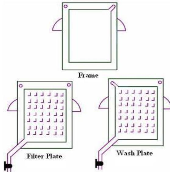
**Fig.9.2 Filter plate and wash plate**
