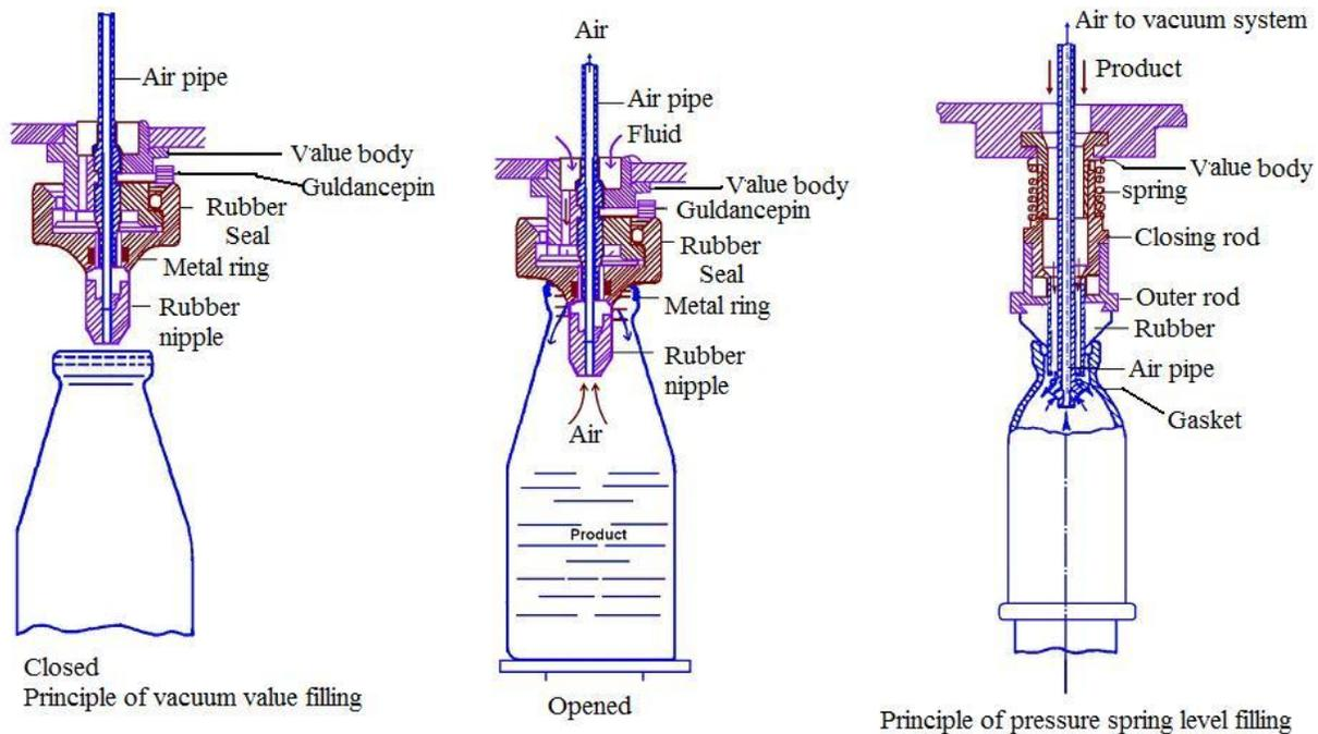
**Fig. 27.1 Vacuum filling of bottles**
