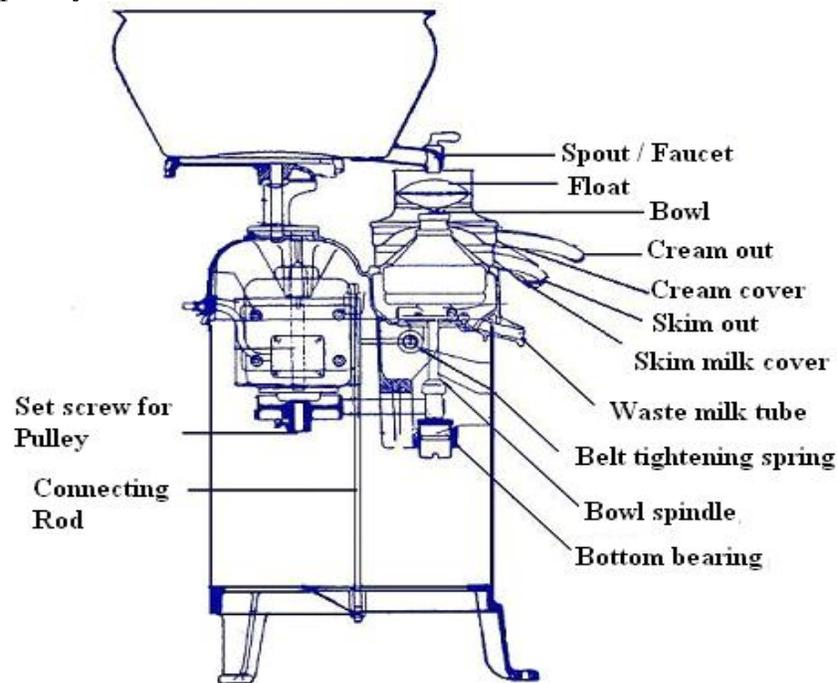
**Fig.11.2 Small capacity cream separator**
