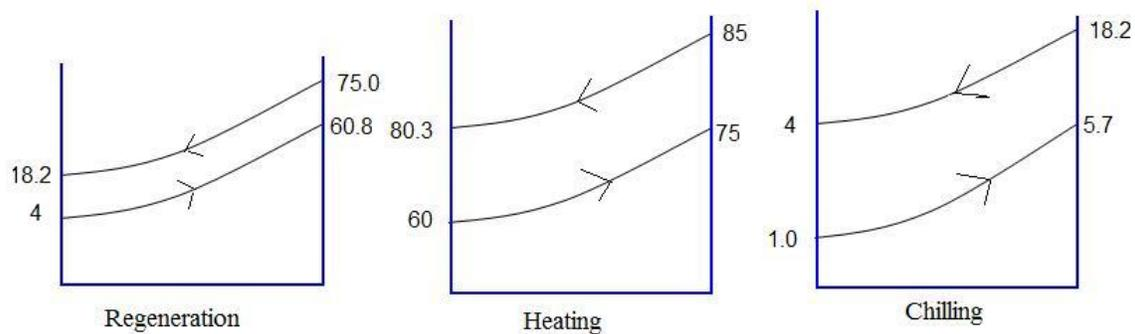
Fig.20.1 Temperature profiles in various section of pasteurizer
