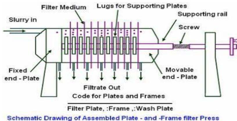
Fig.9.1 Plate and frame filter
