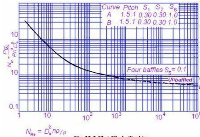
Fig.32.2 Flat-Blade Turbine
