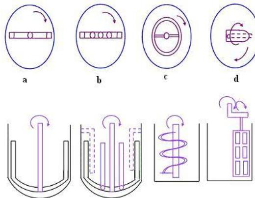
**Fig.30.2 Agitator (Scraping type)**
