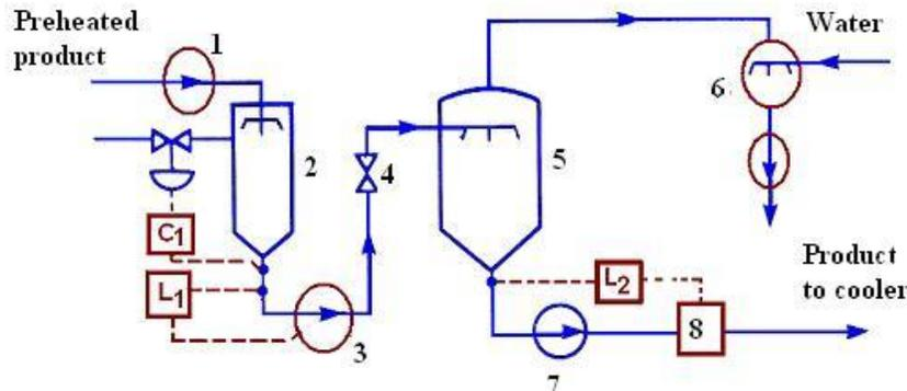
Infusion heating and expansion cooling stage of an Infusion-Type UHT sterilizer
