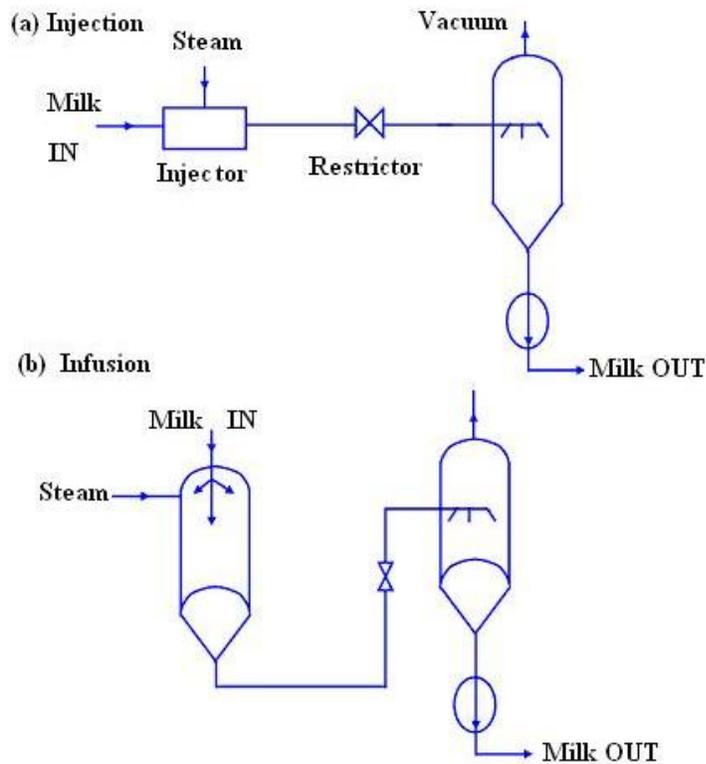
**Fig.23.3 Diagrammatic representation of injection and infusion system**
