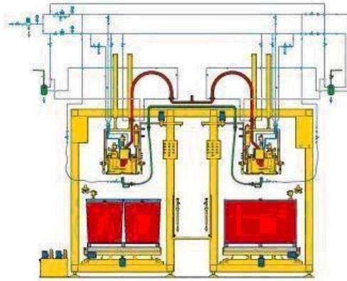
**Fig.29.3 Schematic diagram of bulk filler**
