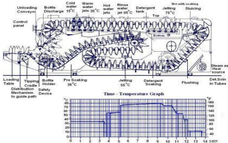
Fig.6.1 Bottle washer (Adopted from Bottle washer manual of Stork company, Holland)
