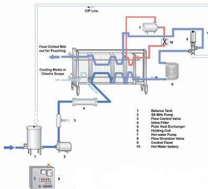
17.2 Schematic diagram of pasteurizer
