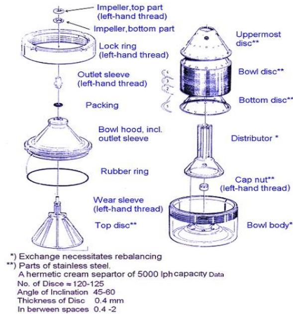
Fig.11.3 Hermetic cream separator (Adapted from Operators manual of Alfalaval Pvt Ltd)
