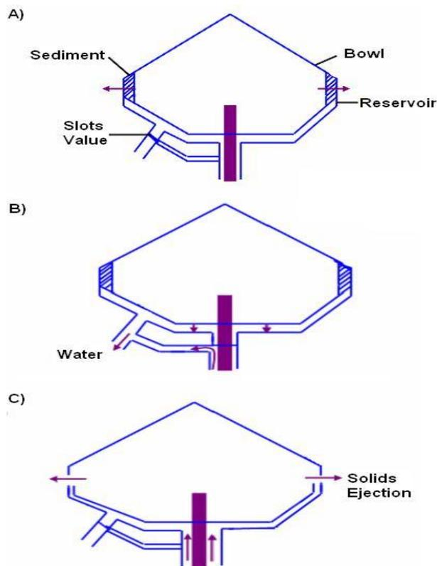
Fig.12.1 Self desludging operation
