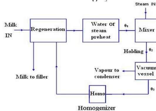
Fig.23.1 Diagrammatic representation of a direct-heating system
