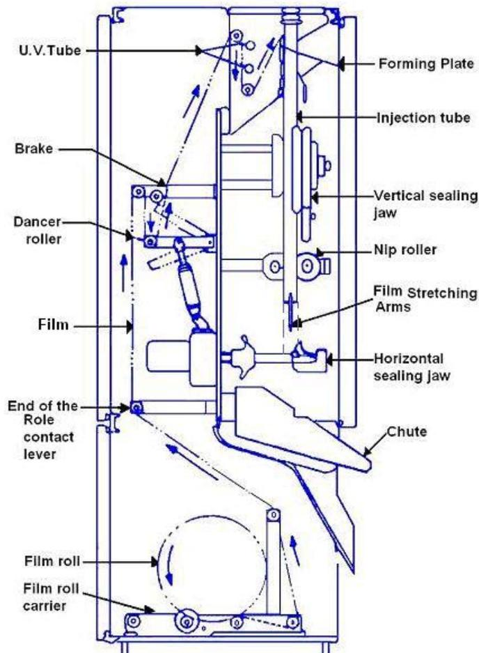
**Fig.28.2 Film feed circuit**
