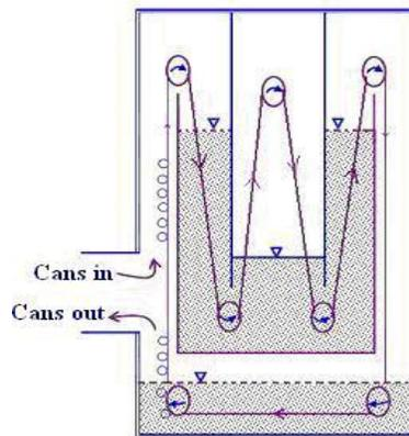
Fig.21.3 Hydrostatic retort
