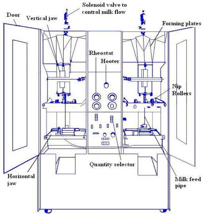
**Fig.28.1 Form-Fill-seal machine**
