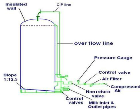
Fig. 4.3 Milk silo tank
