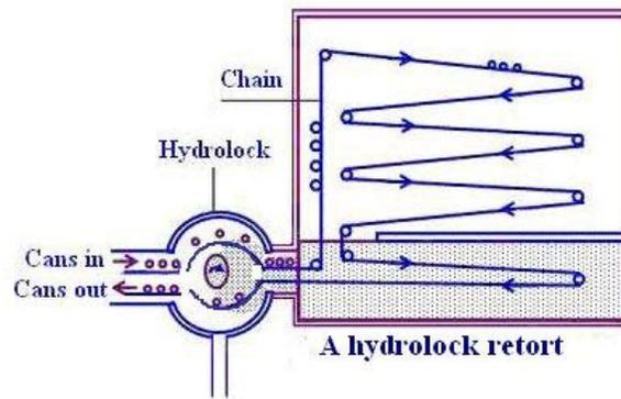
Fig.21.4 Hydrolock retort
