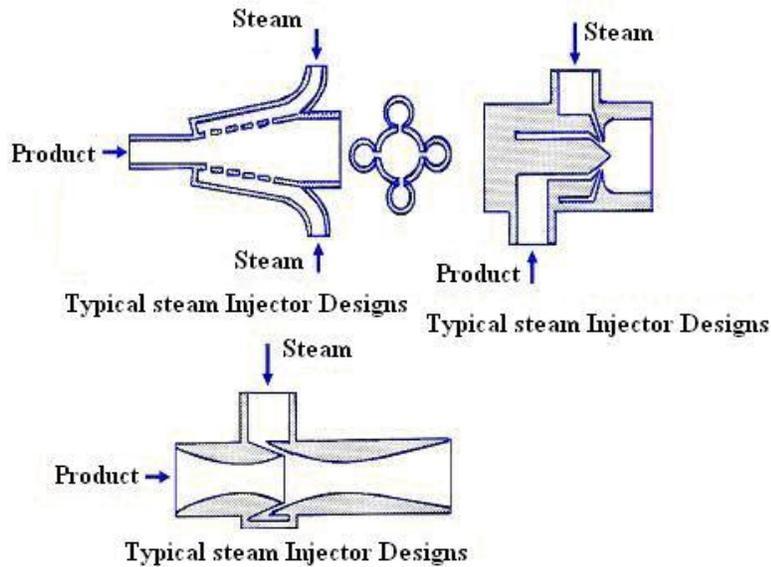
**Fig.23.4 Typical steam injector designs**
