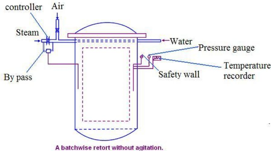
**Fig.21.1 Batch sterilization equipment**
