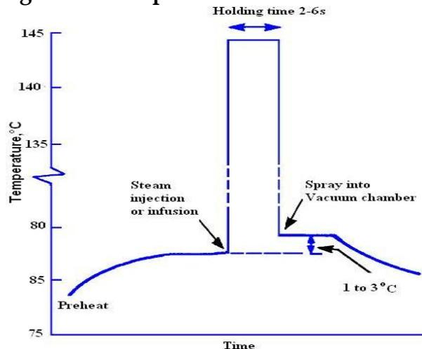
Fig.23.2 Time -temperature relationships during direct heating
