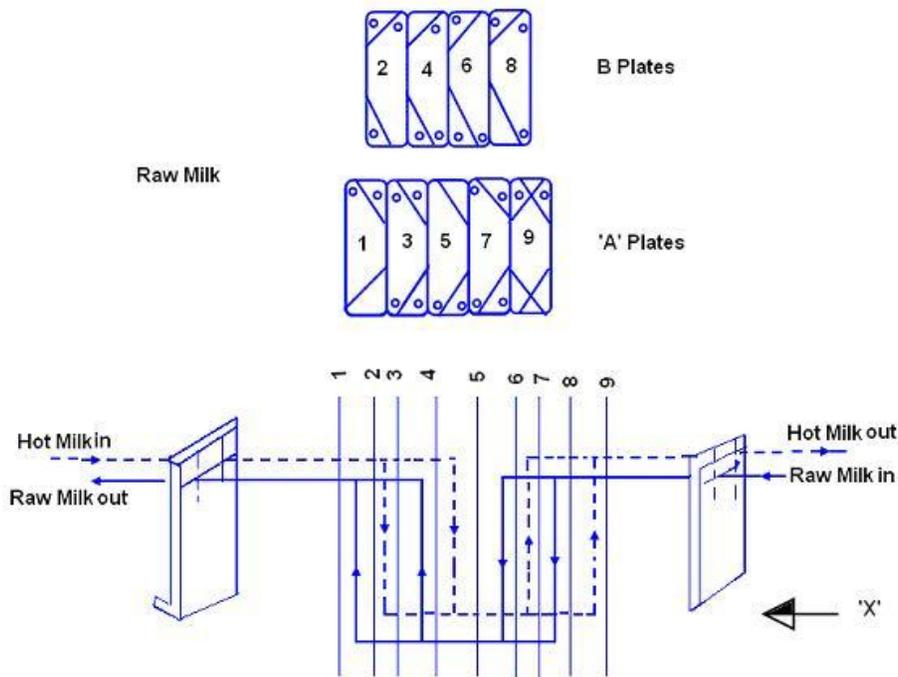
**Fig.17.5 Plate connection diagram**
