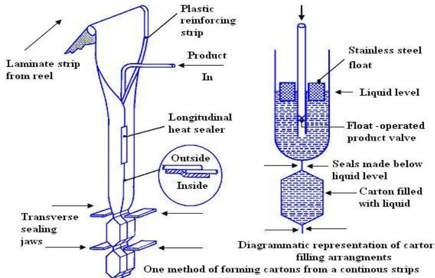
**Fig.24.2 Forming cartons from continuous strips**
