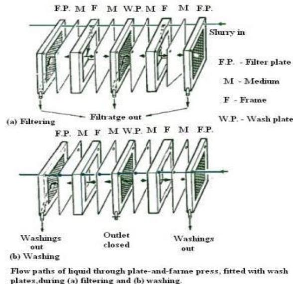
**Fig.9.3 Filtering and washing**
