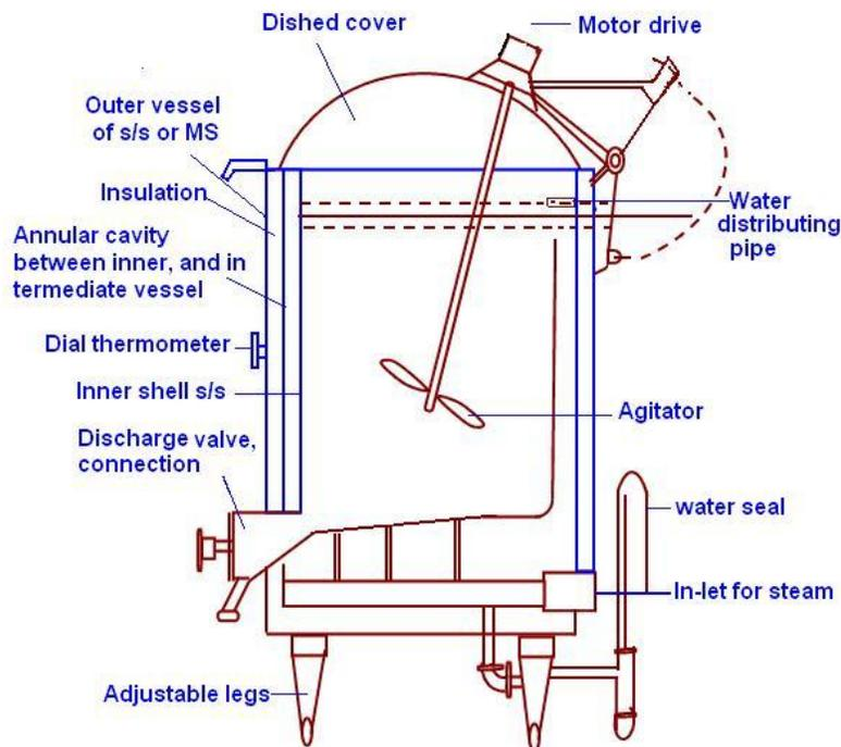
Fig.17.1 Batch pasteurizer
