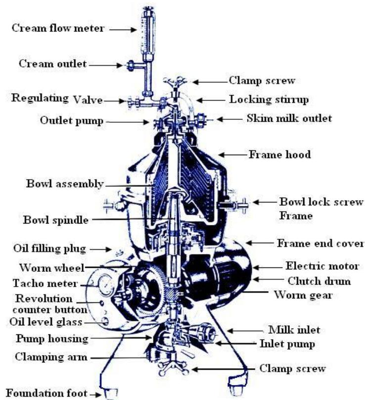
Fig.11.4 Cream separator (Adapted from Operators manual of Alfalaval Pvt Ltd.)
