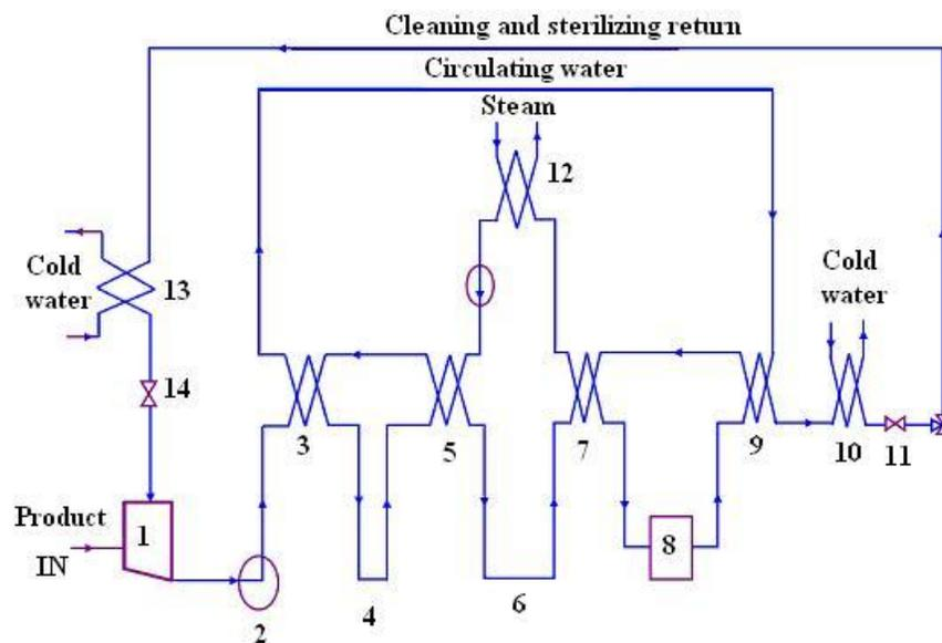
**Fig.22.2 Developed plate-type indirect UHT Plant**
