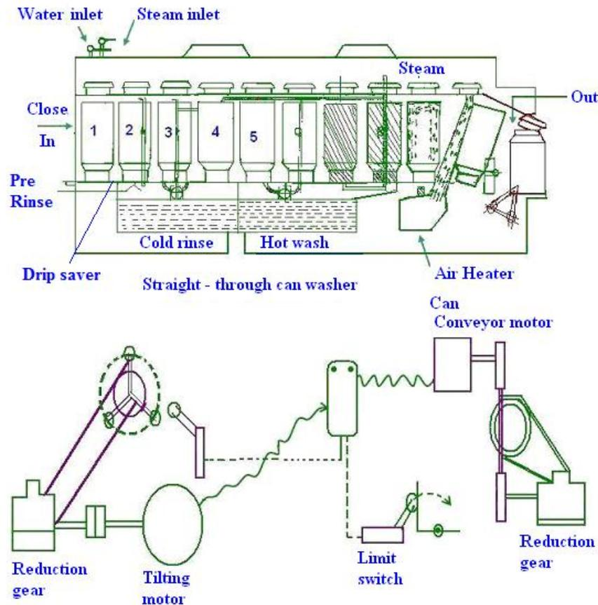
**Fig.5.3 Straight - through can washer**
