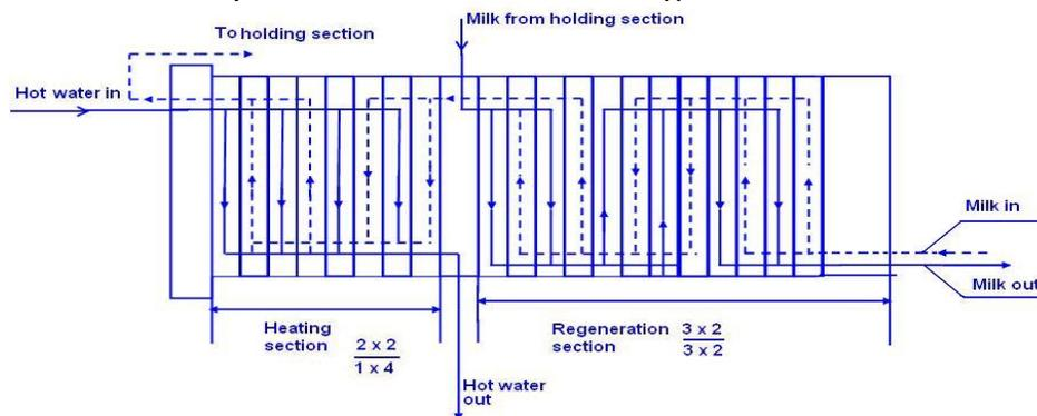
Fig.17.5 Heating and regeneration section
