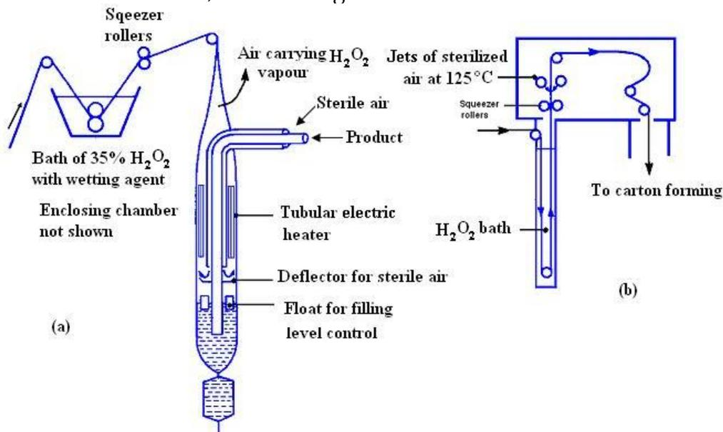
**Fig.24.3 Alternative methods of sterilization of carton material from a reel**
