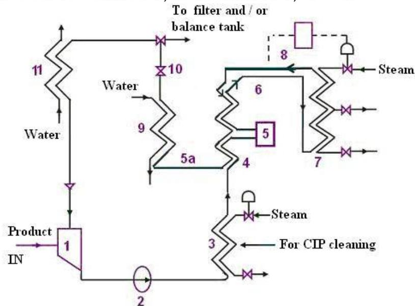
**Fig.22.3 Typical concentric-tube indirect UHT plant**
