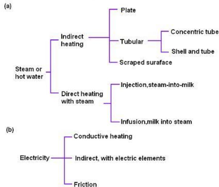
Fig.22.1 Classification of UHT plants and heating energy source
