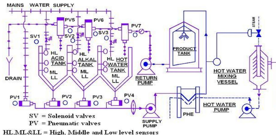
Fig.7.1 Automation of CIP cleaning
