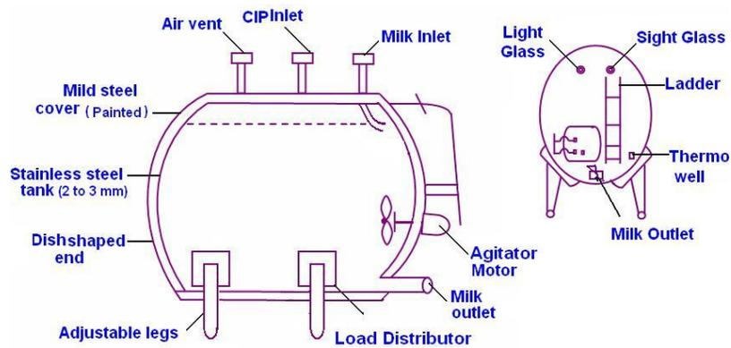
**Fig.4.1 Horizontal milk storage tank**
