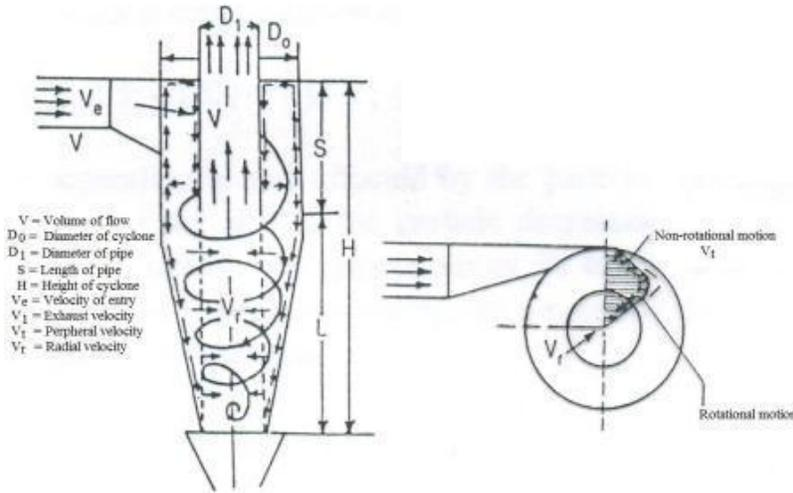
**Fig.8.1 Cyclone separator**
