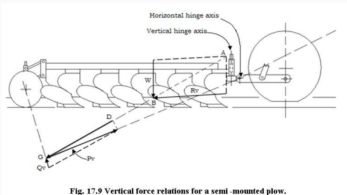
**Fig. 17.9 Vertical force relations for a semi-mounted plow.**
