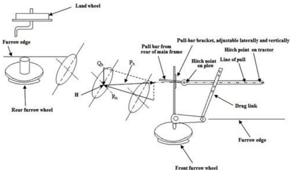
**Fig. 17.2 Horizontal force relations and hitching for a pull-type disc plow.**
