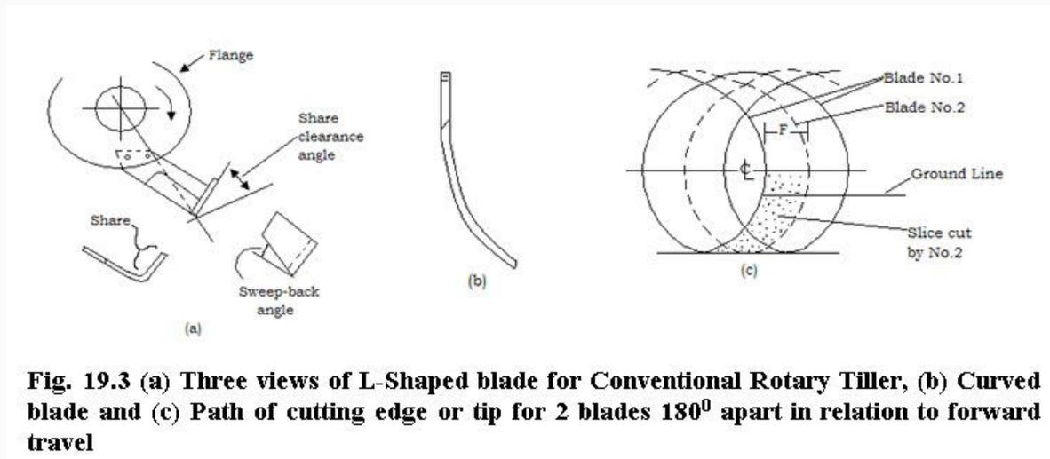
**Fig. 19.3 (a) Three views of L-Shaped blade for Conventional Rotary Tiller, (b) Curved blade and (c) Path of cutting edge or tip for 2 blades 180° apart in relation to forward travel**
