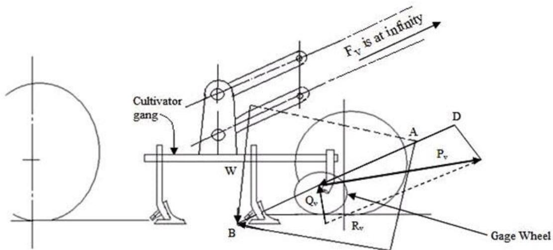
**Fig. 17.12 Vertical force relations for a parallel-link hitch operated as a free-link system**
