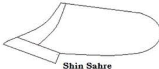
It is similar to slip share with a difference that an extension is provided by side of the mould board.
