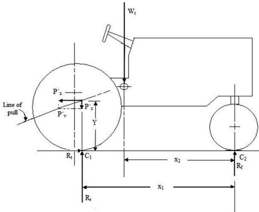
**Fig. 17.10 Vertical force relation for a tractor when pulling an implement at a uniform velocity on level surface**
