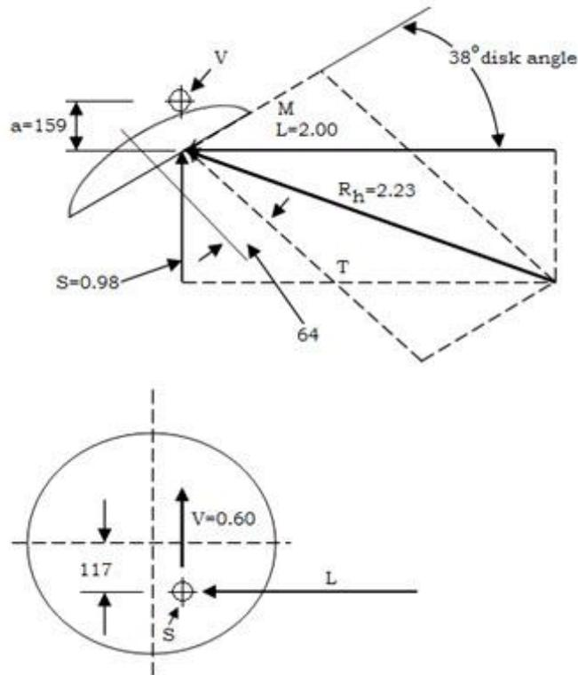
**Fig. 16 (b) Horizontal Force  $R_h$ , plus Vertical Force  $V$**
