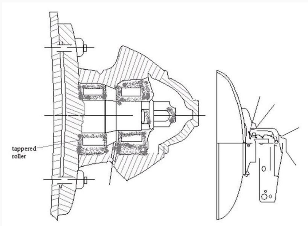
**SCRAPER:** Device to remove soil that tends to stick to working surface of a disc, for great pulverization to furrow slice, invert the furrow slice and cover the trash better.
