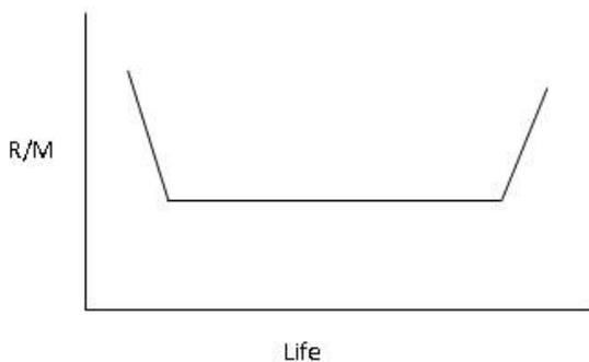
Also called bath-tub curve. Firstly repair and maintenance is less than because constant offer that start increasing i.e. the time to buy a new machine.
