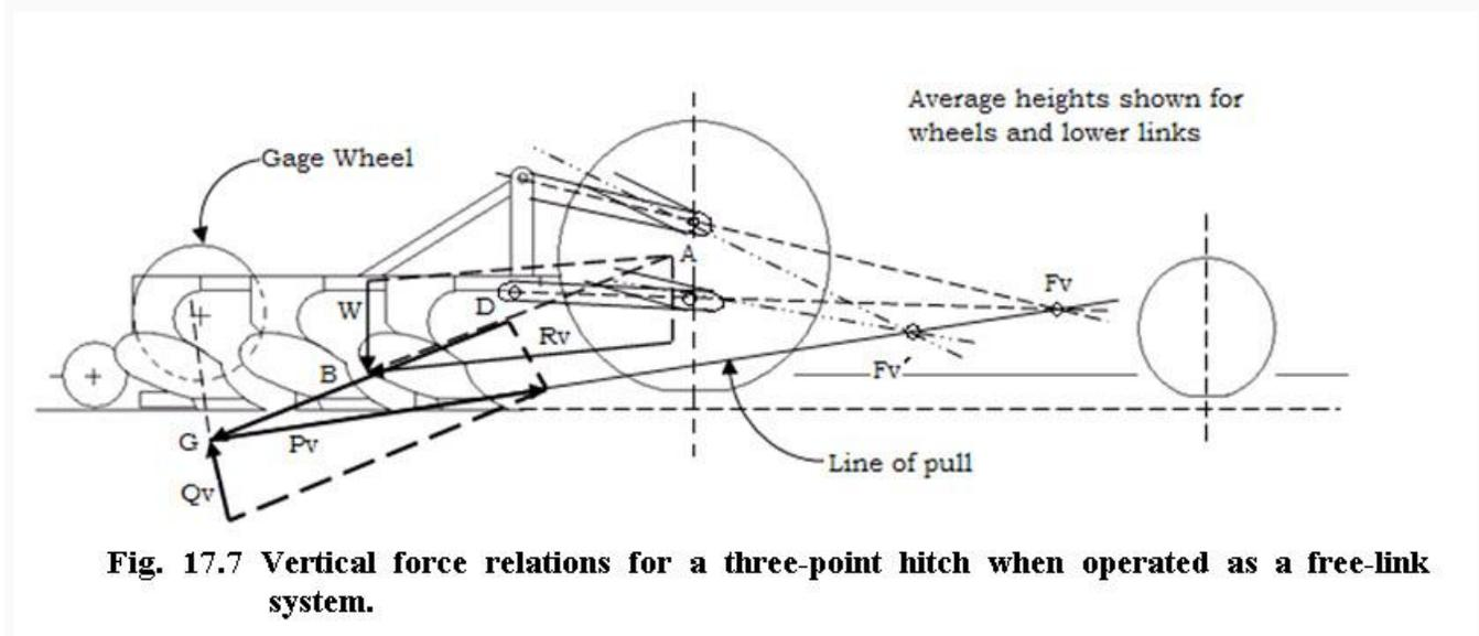
**Fig. 17.7 Vertical force relations for a three-point hitch when operated as a free-link system.**
