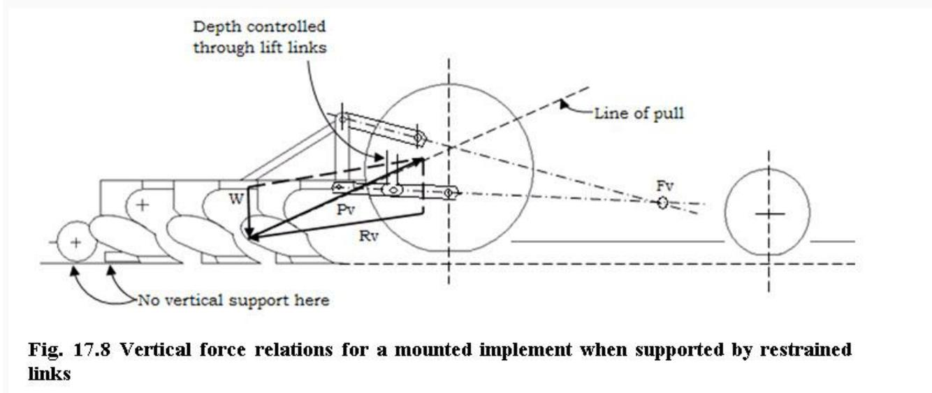
**Fig. 17.8 Vertical force relations for a mounted implement when supported by restrained links**
