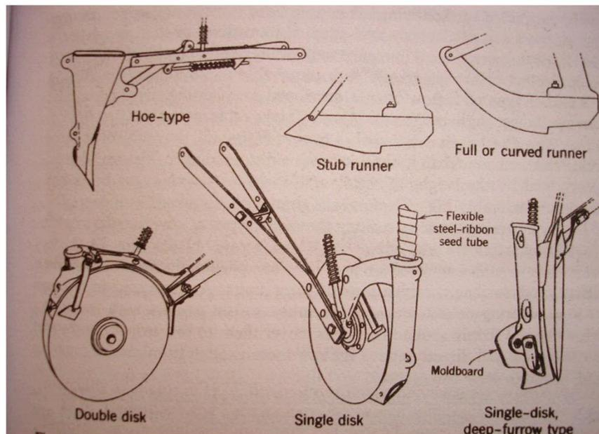
**a) Hoe Type:** They are equipped with spring tips and suitable for stony or root-infested soils. They are similar to shovel type and also used for deep placement of seeds if soil is relatively free of trash.
