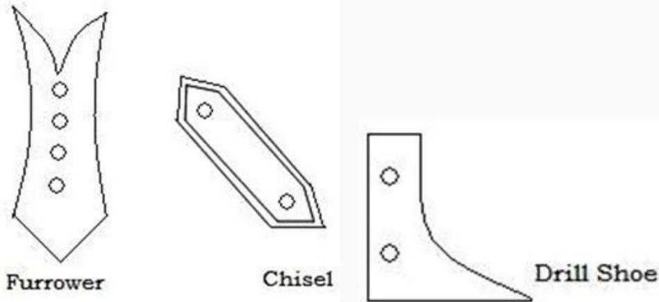
Drill shoe is used for sowing purposes, furrower and sweep for Intercultural.
