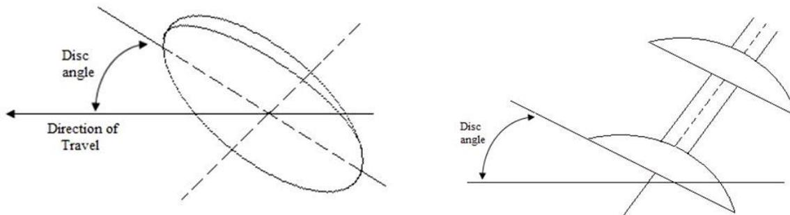
**TILT ANGLE:** It is the angle at which the plane of cutting edge of disc is inclined to vertical line. Tilt angle varies from 15 to 25 degree.
