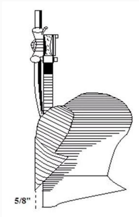
REACTION OF SOIL TO MOULD BOARD: Wide range of soil conditions encountered in tillage materially affects the reactions of the soil on mould board surfaces.
