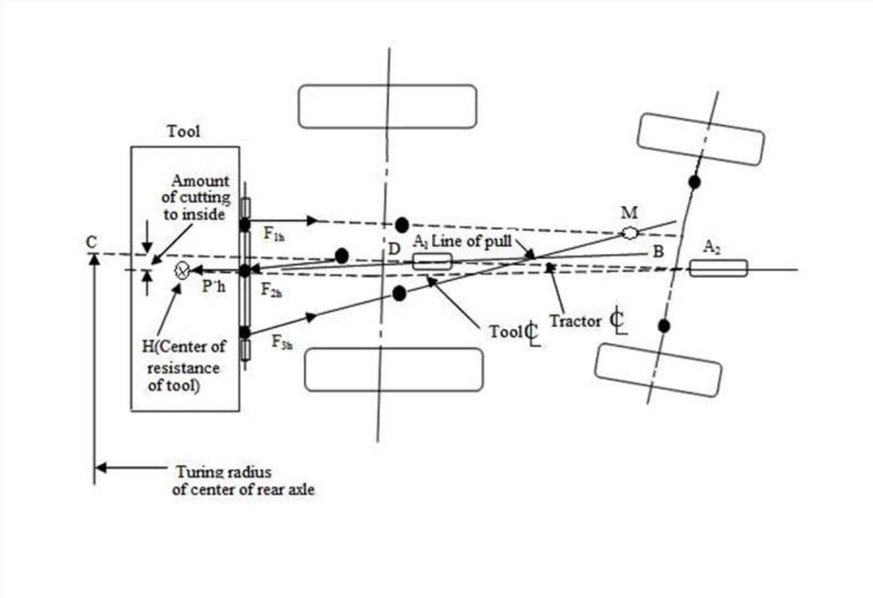
**Fig. 17.11 Testing characteristics with horizontally converging pivotal links (three-point hitch) while operating around a curve**
