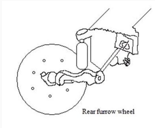
(5) Bearings: Disc blades are at an angle to the direction of travel so both radial and thrust forces are present. Radial forces push against an axle at right angle while thrust forces push along the axis. That is why taper roller bearings are used.
