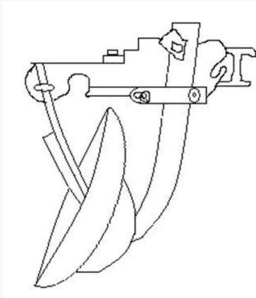
(2) Standard: Connects disc bearing and plough frame. Sometimes beam is bent for disc attachment for reducing the cost.
