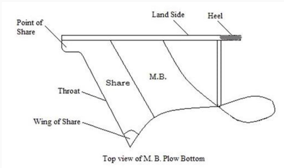
a) Share: It is the part of plow bottom which actually penetrates into the soil and makes a horizontal cut below the surface.
