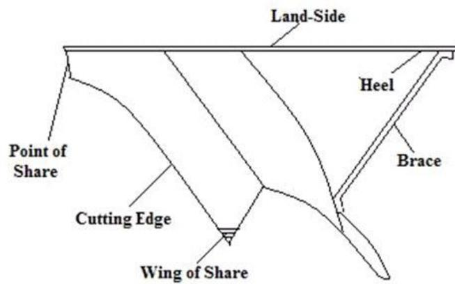
3) **Angle of cutting edge** from direction of travel it is 40-45 degrees.
