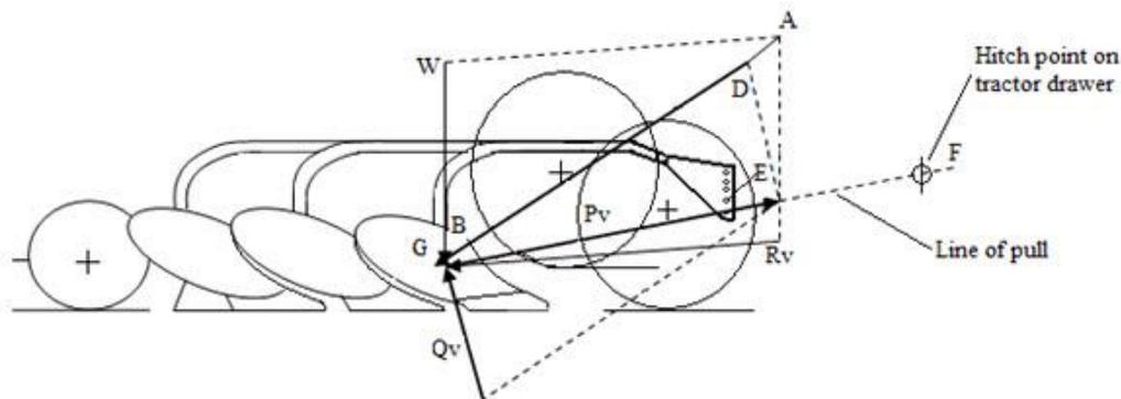
**Fig. 17.3 Vertical force relation for a pull type mould board plough having support wheels and hinged pull members**
