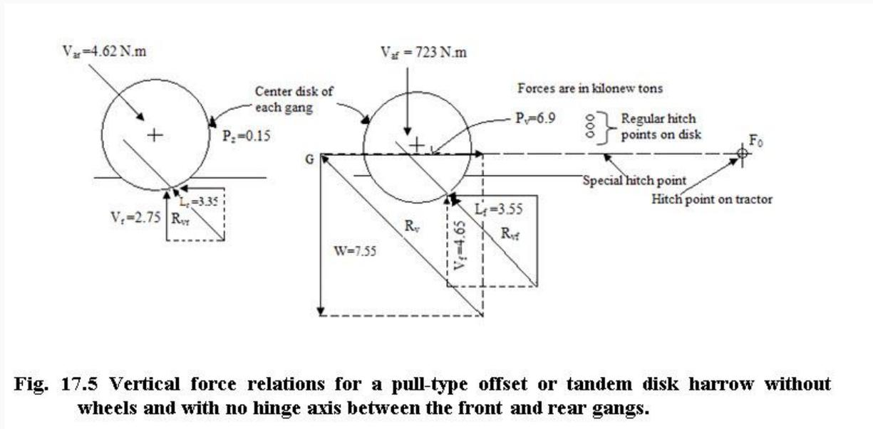
**Fig. 17.5 Vertical force relations for a pull-type offset or tandem disk harrow without wheels and with no hinge axis between the front and rear gangs.**
