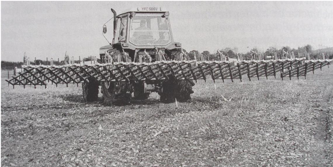
**Fig. Fully mounted hydraulically controlled 9-m straight-tined harrow**
