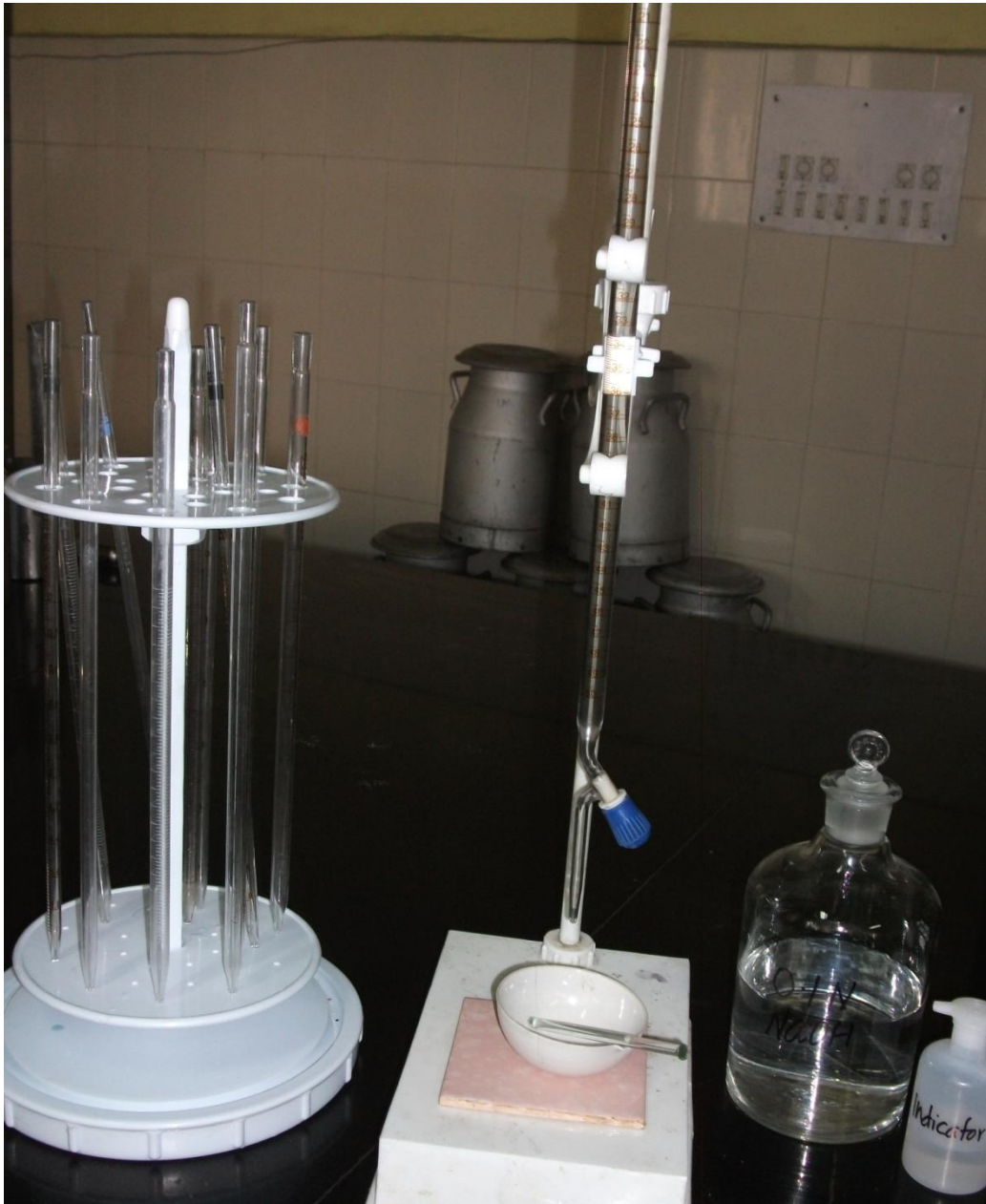
Fig. 43.3 Acidity checking assembly
