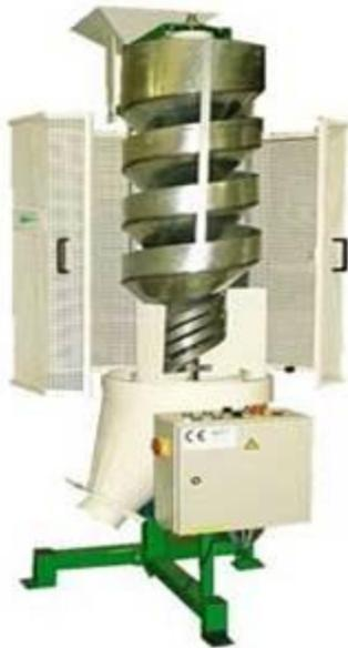
The orbit of round seed increases with speed on its flight around the axis, until it rolls over the edge of the inner flight into the outer flight where it is collected separately. The slower moving seed does not build up enough speed to escape from the inner flight. Most spirals have multiple inner flights arranged one above the other to increase the capacity.
