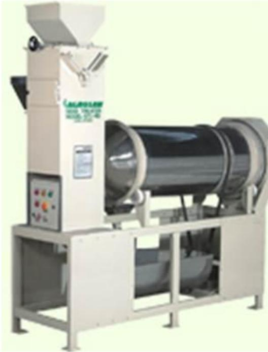
Slurry tanks have 15 to 35 gallon capacities, depending upon the size of the treater. They are equipped with agitators that mix the slurry in the tank and keep it suspended during operation. It is important that the powder be thoroughly suspended in water before treating. If the treater has been idle for any period of time, sediment in the bottom of the slurry cups must be cleaned out.
