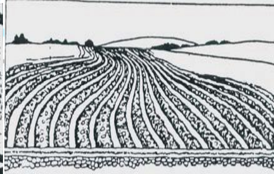
Fig. 5.4 Graded contour-furrow Irrigation
