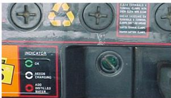
Fig: 8. View of battery from top side showing indicator systems
